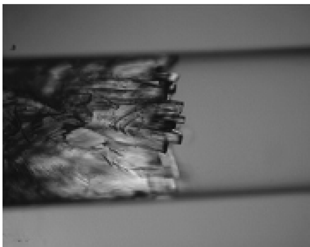
Fig. 1 Crystals of alpha-amylase grown (a) in microgravity and (b) in terrestrial. The diameter of the capillary is 0.5 mm.
